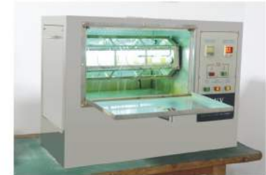
Anti-uv Tester Plastic parts test, how long its color will be changed.
