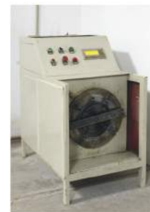
Spring Fatigue Tester Coil spring life test.
