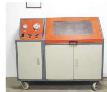
Bursting Tester Burst pressure test of hose and complete machine.
